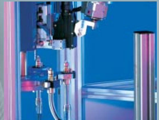
4 Rotor carousel rotates a replacement neck into position.
