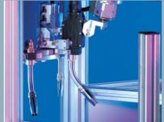
2 Neck release mechanism is engaged and wire is cut inside the torch body.
