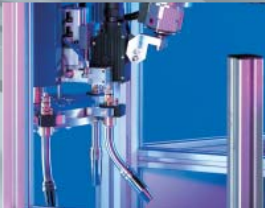
3 The change neck is taken off by the downward movement of the rotor plate. Quick release valves in the water channels avoid leaking of the coolant.
