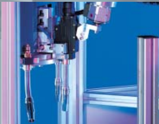
5 Replacement neck is locked into position. All supply connectors are automatically made, robot moves out of change station and continues.
